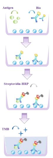
1. Add 50  $\mu L$  standard or sample to the wells, immediately add 50  $\mu L$  Biotinylated Detection Ab Working Solution to each well, incubate at 37°C for 30 minutes
