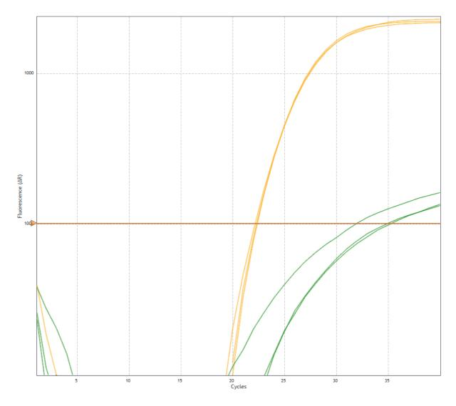
*Low pork signal in the FAM fluorescence channel Positive IPC (Internal Positive Control) signal in the ROX fluorescence channel*
