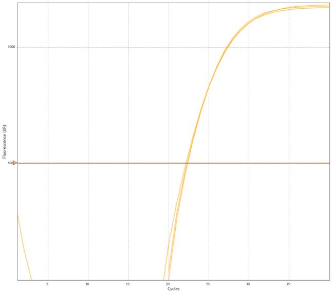
*No / negative pork signal in the FAM fluorescence channel Positive IPC (Internal Positive Control) signal in the ROX fluorescence channel*
